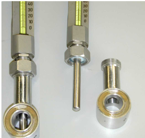
Figure 3.4 Traditional temperature sensor with unacceptable dead end.
