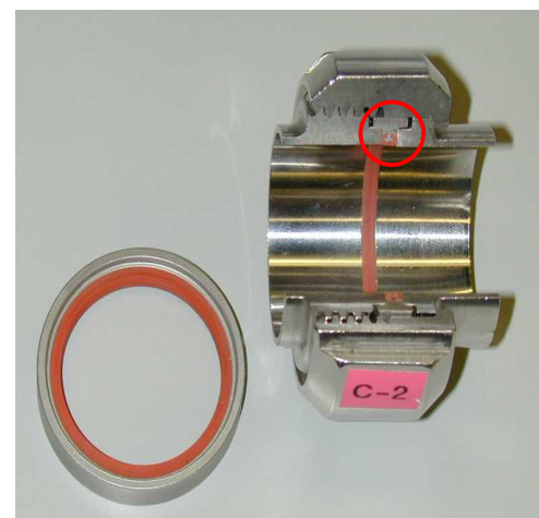
Figure 3.28 ISO 2853 coupling with T-gasket (red circle) that improves alignment and controls compression of the gasket.
