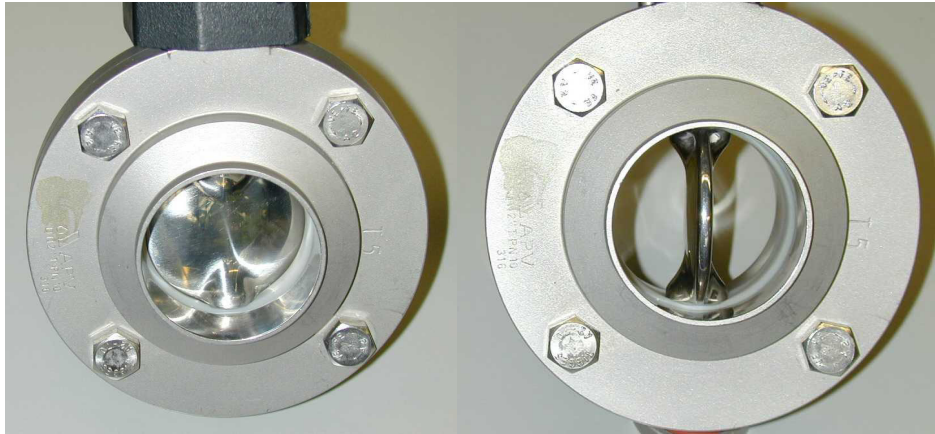
Figure 3.19 Butterfly valve in closed and open position.
