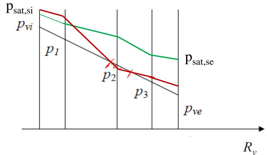
$$g_v = \frac{(p_{vi} - p_{ve})}{R_v} \quad \text{kg} / \text{m}^2 \text{s}$$
