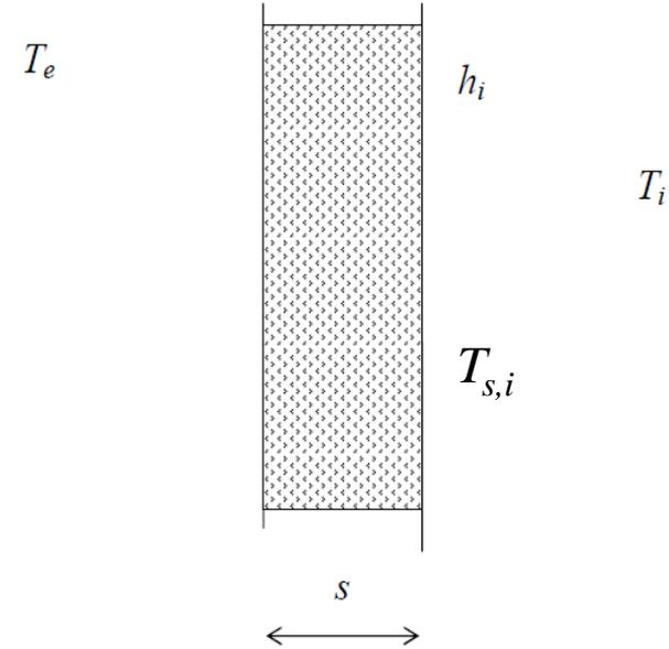
$$q = \frac{T_i - T_e}{R} \quad \text{con} \quad R = \frac{1}{h_i} + \sum_{j=1}^n \frac{s_j}{\lambda_j} + \frac{1}{h_e}$$
