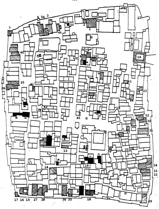
Plan of the old city of Shibam indicating the buildings which are decayed or damaged (Nos.! to 48) and those which are ruins (Letters A to M).
