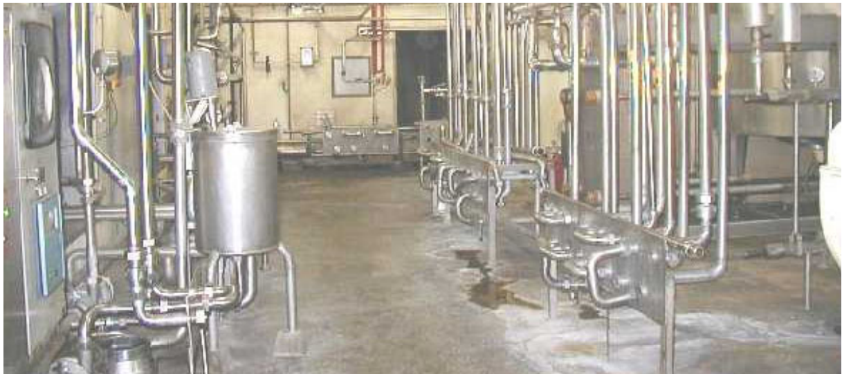
Figure 2.12 Water and residuals of NaOH on floor which can cause a damaged floor.
